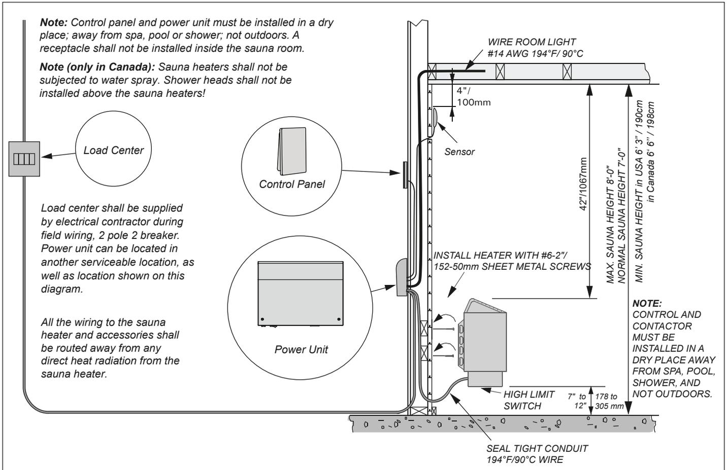
Figure 1. Digital Sauna Control CX170-U1 and CX170-U3
