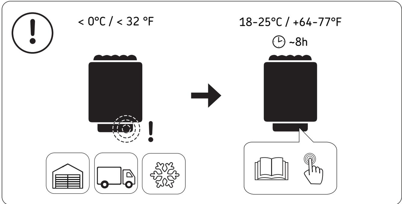
**!** Overheat protector of the device can also go off at temperatures below  $-5^{\circ}\text{C}$  /  $23^{\circ}\text{F}$  (storage, transport, environment). Before installation take the device to a warm environment. The overheat protector can be reset when the temperature of the device is approx  $18^{\circ}\text{C}$  /  $64^{\circ}\text{F}$ . The overheat protector must be reset before using the device. See the user manual > Resetting the Overheat Protector.
